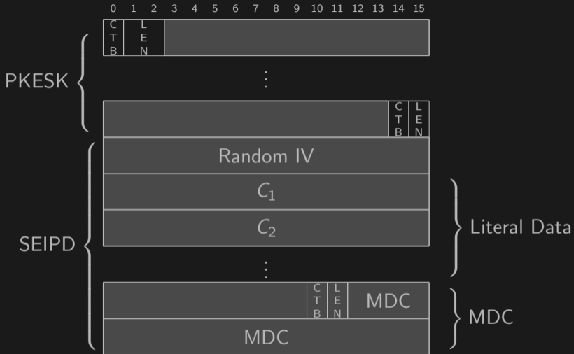
Figure 15: OpenPGP packets structure
