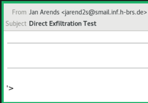
Figure 18: Direct exfiltration attack in Thunderbird 52.9
